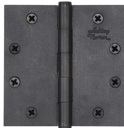
HIN4545 Shown in dark bronze patina 4 1/2" x 4 1/2" 0.134" thickness Supplied with #12 x 1 1/4" screws
