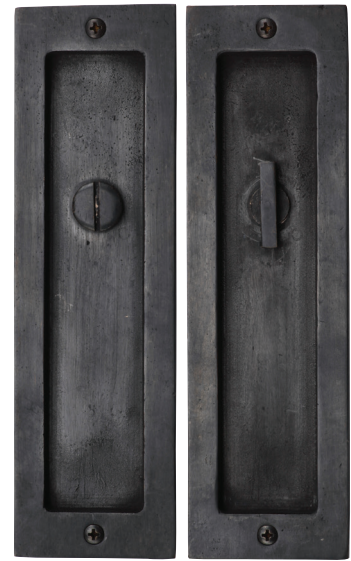
Sliding/Pocket Door Hardware 8 1/2" x 2 1/2" Shown in dark bronze patina Supplied with Accurate mortise lock Minimum door thickness 1 3/4"
