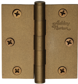
HIN3535 Shown in light bronze patina 3 1/2" x 3 1/2" 0.123" thickness Supplied with #10 x 1" screws
