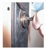
Insert key halfway into cylinder and thread cylinder into housing until it is against the trim and does not interfere with the swing cover.
